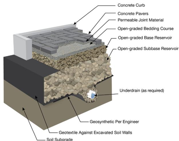
Figure 1. Typical permeable interlocking concrete pavement cross section.
