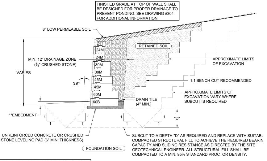
\*\*EMBEDMENT SHOULD BE THE GREATER OF 6" OR H/20 FOR WALLS WITH LEVEL GRADE AT THE TOE. REFER TO RECON'S EMBEDMENT RECOMMENDATION DOCUMENT FOR ADDITIONAL INFORMATION FOR WALLS WITH A TOE SLOPE CONDITION.
