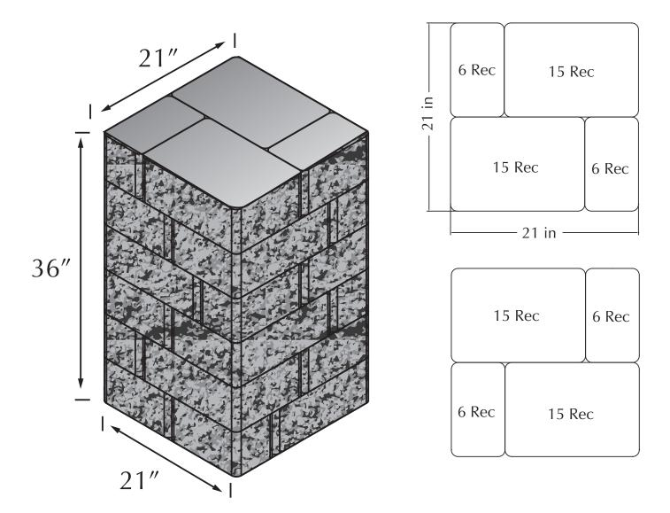
Each column is 21" x 21" square. There are 24 pieces of each sized block on the pallet for a total of 48 blocks. The kit will make two (2), 3-foot tall columns.
