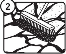
Using the street broom, fill joints completely. Spread NOCO™ over **short distances**.
