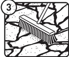
Remove excess NOCO™ from the surface with the broom.
