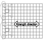
Geogrid is to be placed on level backfill over the fiberglass pins. Place next unit. Pull grid taut and backfill. Stake as required.
