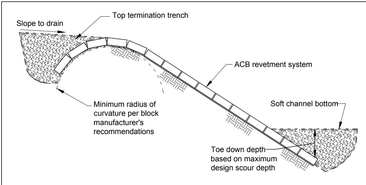
Figure 7.6: Conceptual detail of minimum radius-of-curvature for bank protection.
