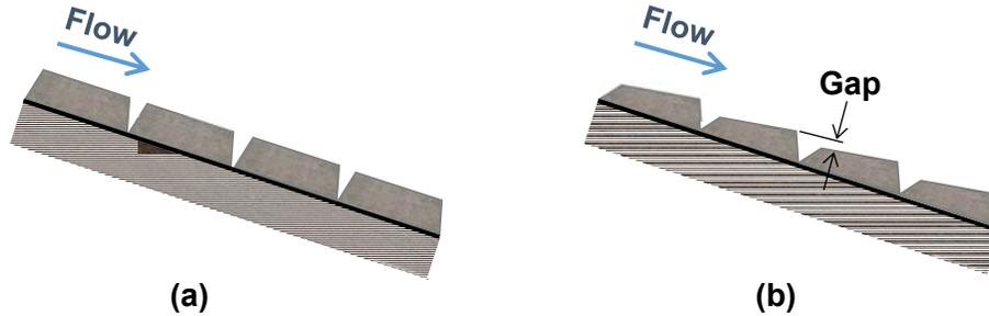
Figure 2.10: Profile view of block system illustrations: (a) untapered block system and (b) tapered block system (dimensions are exaggerated for illustration).
