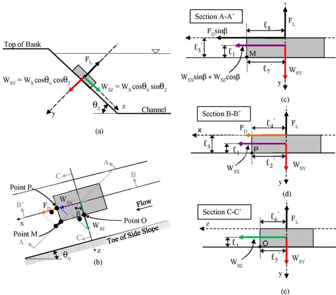
Figure 4.1: Force diagrams for safety factor analysis: (a) cross-section view normal to bed slope, (b) view normal to side slope, (c) rotation about Point M along Section A-A', (d) rotation about Point P along Section B-B', and (e) rotation about Point O along Section C-C'.
