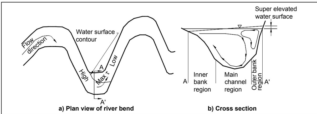
Figure 2.1: (a) Plan view of a river meander bend with region of increased shear stress indicated (b) Cross section A-A' illustrating super elevation at outer bank of the bend.
