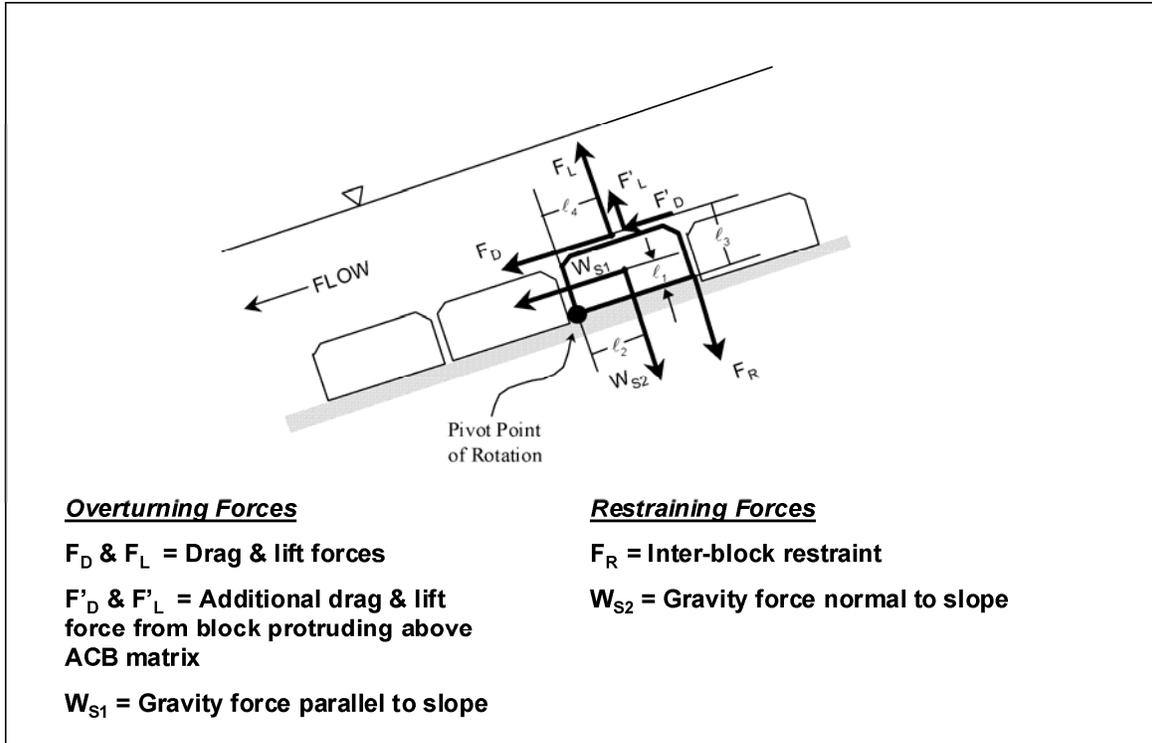
Figure 2.6: Moment balance on an ACB at incipient failure.
