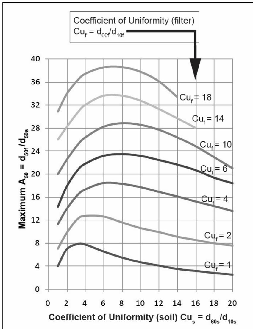
Figure 5.6: Granular filter design chart according to Cistin and Ziems (ref. 37).
