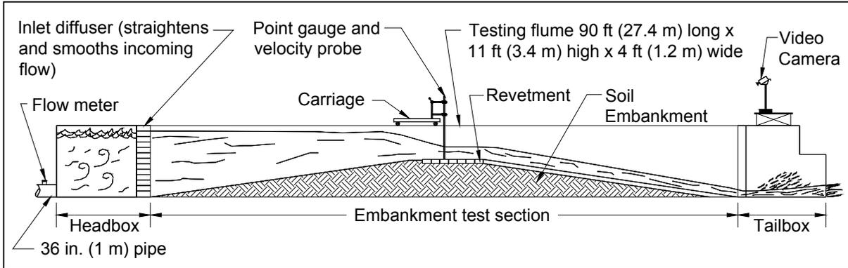
Figure 2.7a: Schematic of a typical laboratory flume for ACB performance testing.
