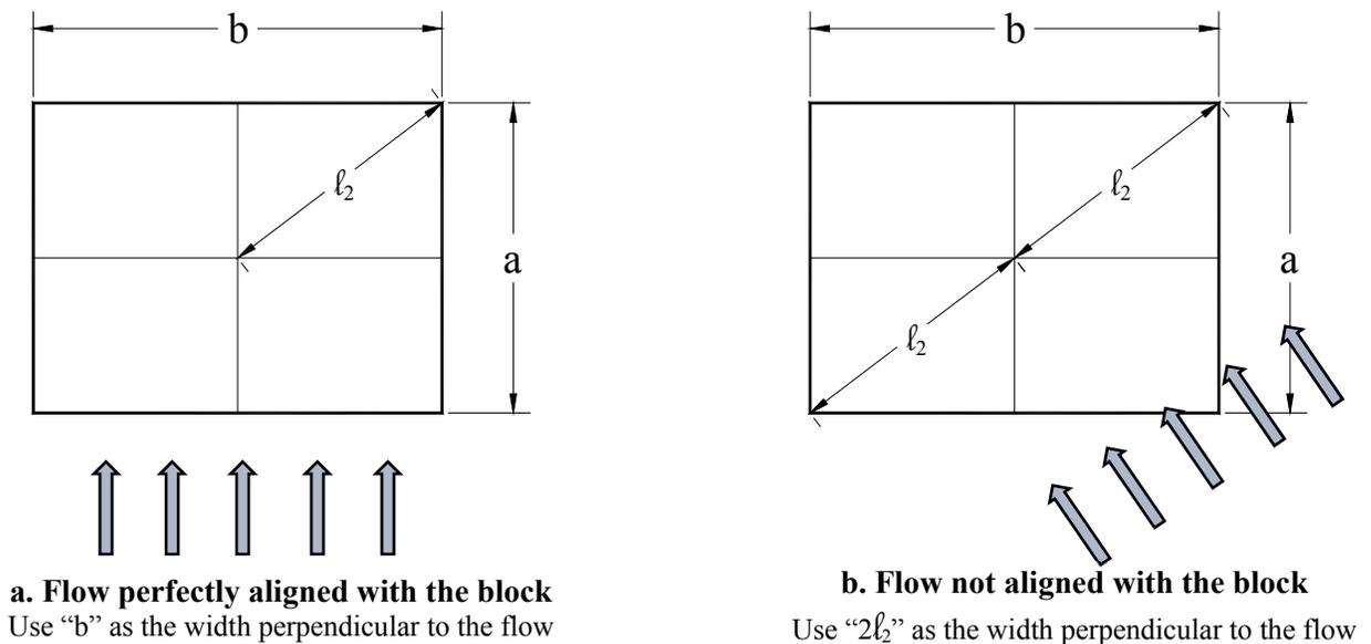
Figure 2.9: Block dimensions and flow direction.
