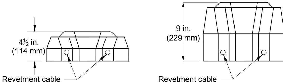
**Figure 2.8:** Comparison between the potential intra-block friction between 4.5 in. (114 mm) and 9.0 in. (229 mm) ACB units. (Courtesy of Submar, Inc.)
