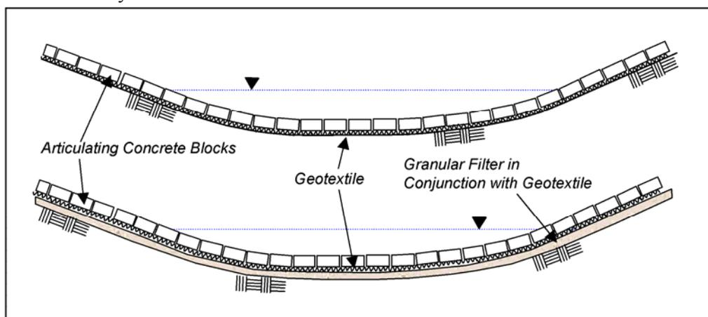
Figure 5.1: Channel cross-sections showing filter and bedding orientation.
