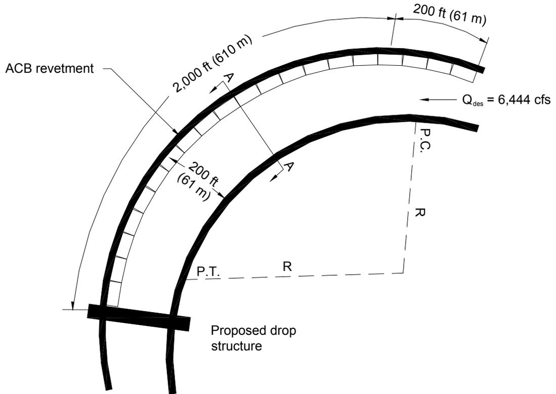
(A) Plan view of problem setting and ACB system installation
