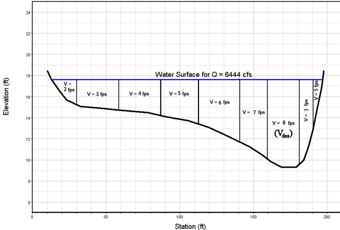
Figure 3.4: Velocity Distribution at Critical Cross-Section from HEC-RAS Model.
