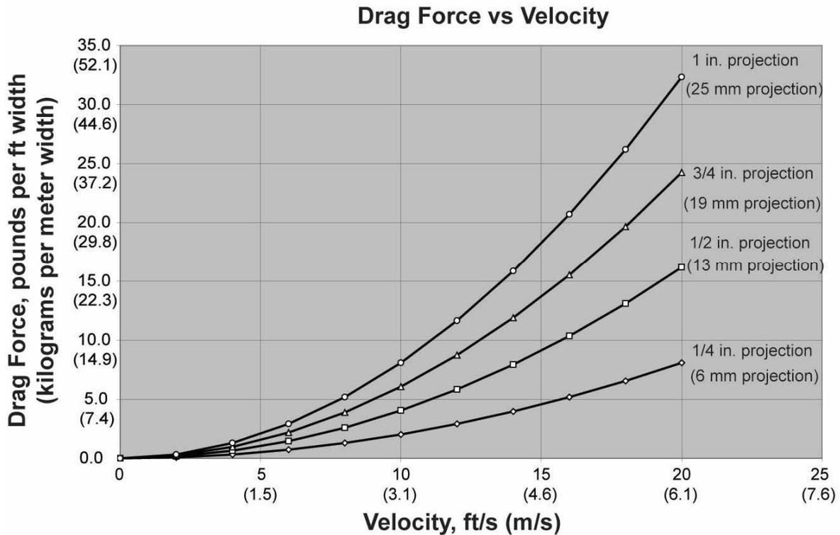
Figure 2.5: Relationship between drag force, velocity and protrusion height
