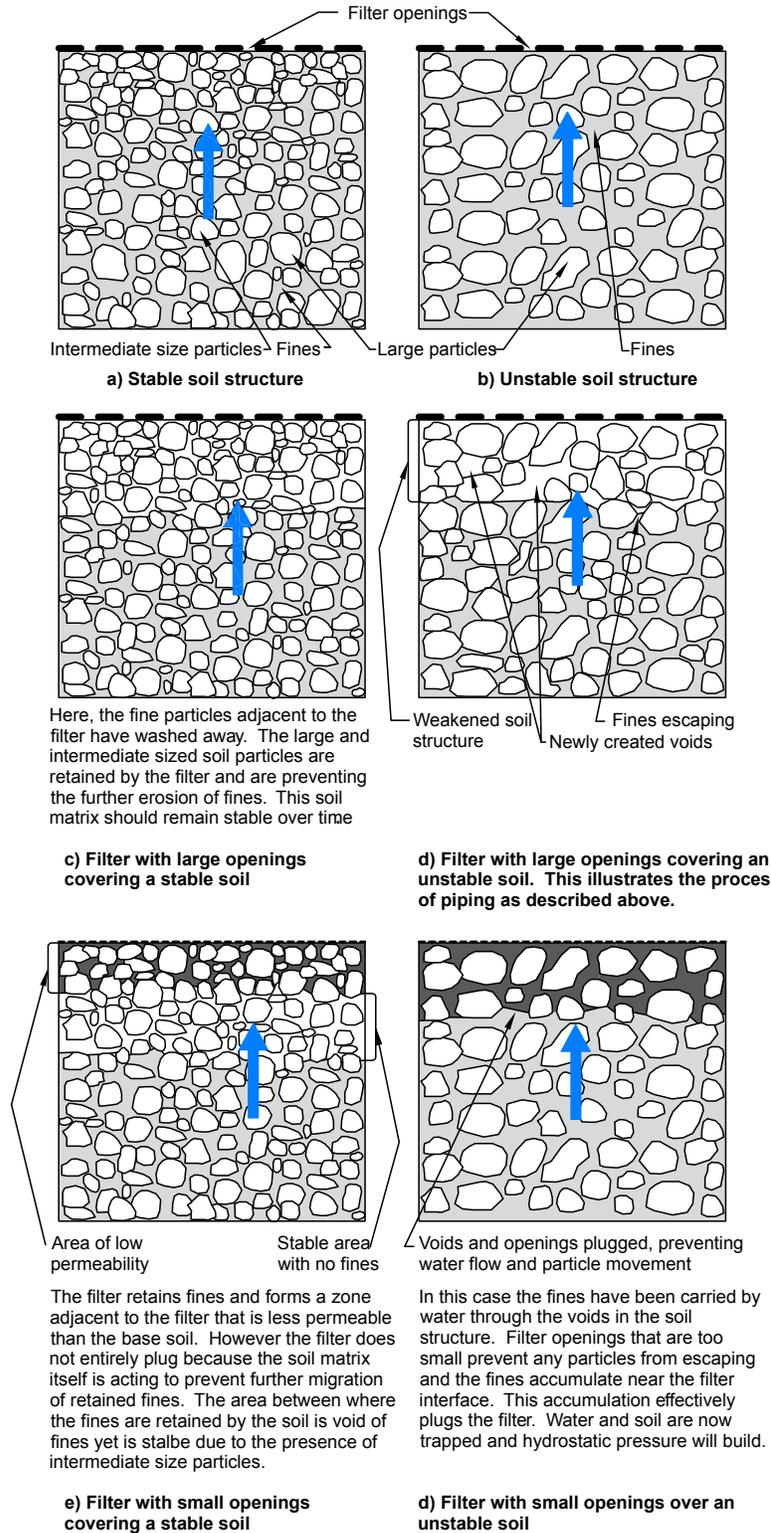
Figure 5.2: Examples of soil and filter subgrades.
