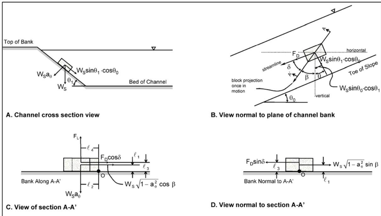
Figure 3.1: Three-dimensional view of a block on a channel side slope with factor of safety variables defined.
