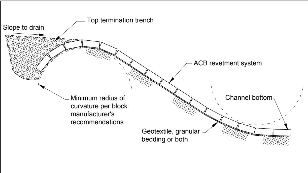
Figure 7.4: Conceptual detail of minimum radius-of-curvature for bed and bank protection.
