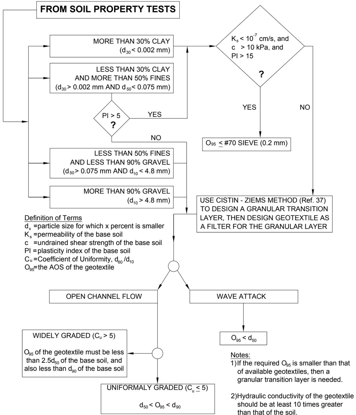
Figure 5.5: Geotextile selection based on soil retention (ref. 37).
