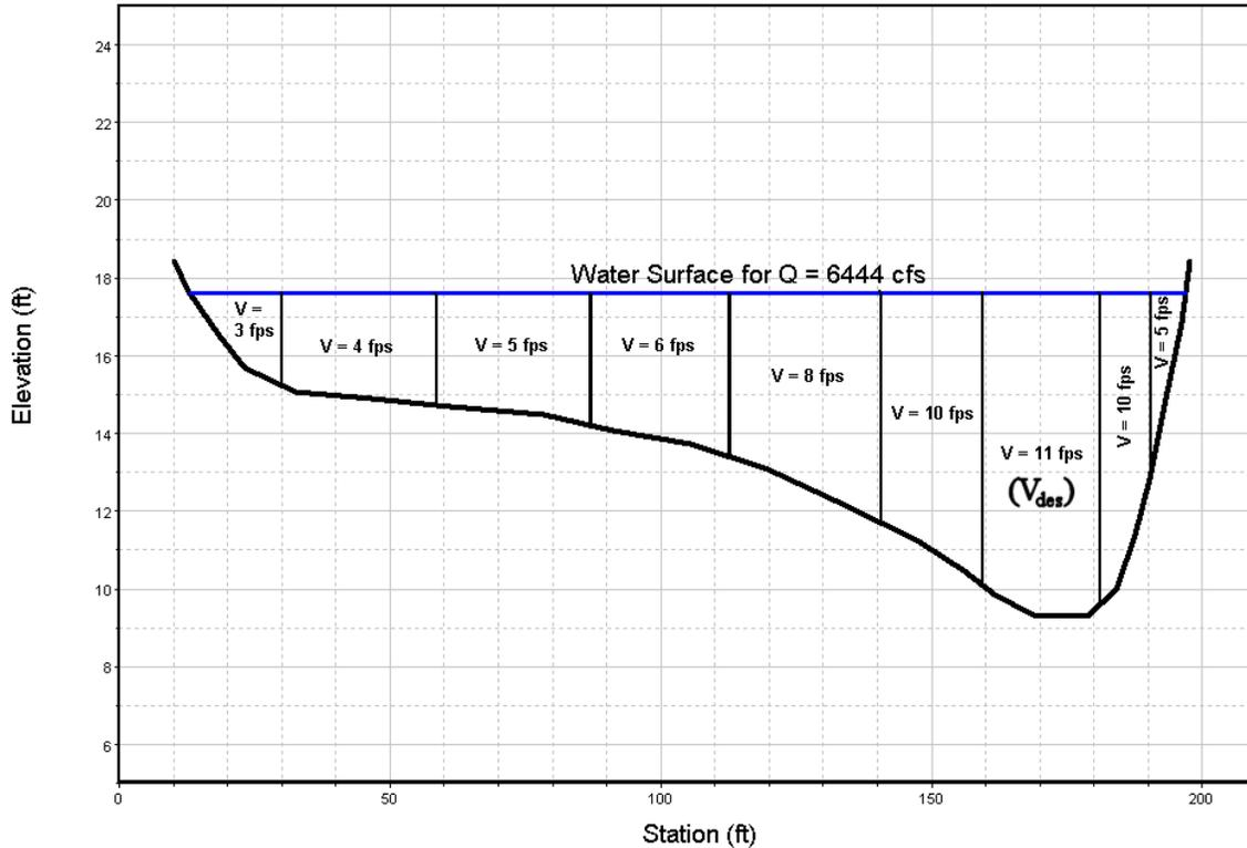
Figure 4.3: Velocity Distribution at Critical Cross-Section from HEC-RAS Model.
