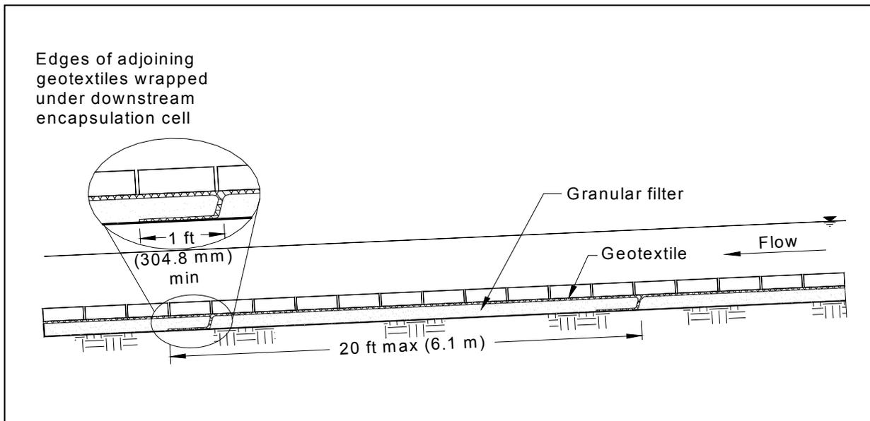
Figure 7.1: Granular filter detail showing granular filter encapsulation.
