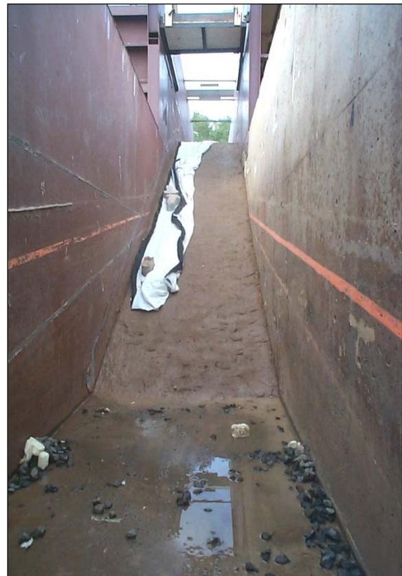
Figure 2.7c: Photograph of subgrade inspection after a series of full-scale tests (courtesy of Colorado State University).
