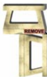
Remove notch to form corner
